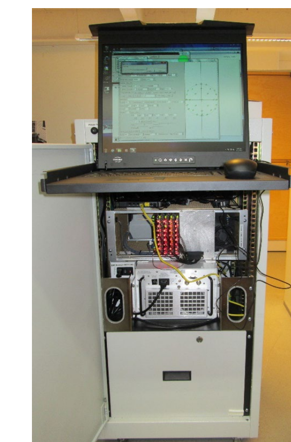
SMS-EIT clinical prototype (left); Independent channels enable generation of current patterns to optimally measure impedance within the body (right)
